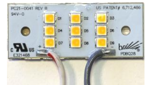
LED module with MCPCB and 3mm LED
