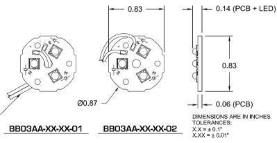
Ts measurement point is cathode of any LED
