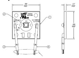
Entire top of module is conformal coated with Humiseal 1B31 or equivalent
